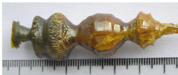
Fig. 1. Lead tungstate crystal obtained by pulling from melt, using kanthal wire instead of a seed crystal (as a consequence, the intense coloration due to impurification).
