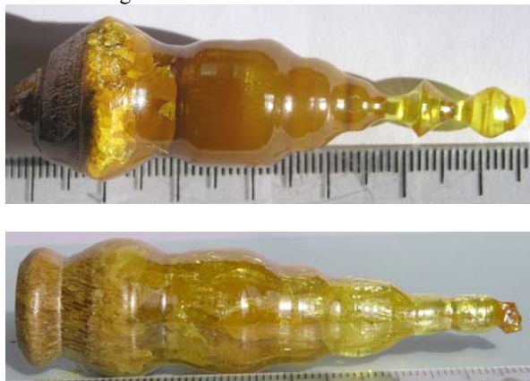
Fig. 2. \text{PbWO}_4 crystals obtained after repeated pullings from selected crystalline material (the clearer upper part, free of paramagnetic impurities, is evidenced).
