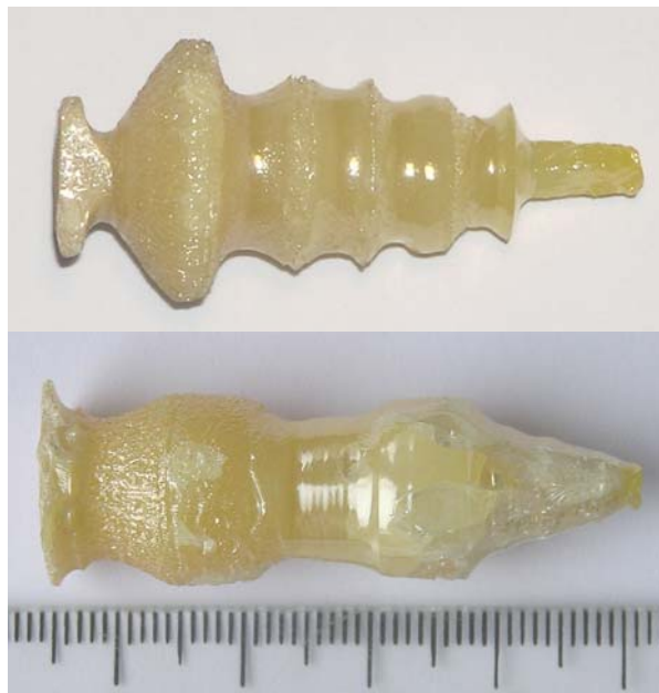
Fig. 3. \text{PbWO}_4 crystals obtained from ultrapurified starting materials (single crystals of \text{Na}_2\text{WO}_4 and \text{Pb}(\text{NO}_3)_2 , grown from aqueous solutions).
